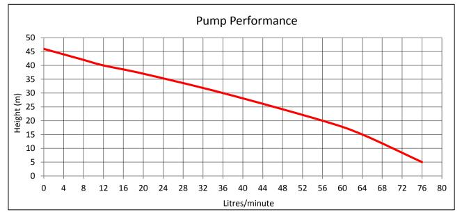
NOTE: The above Performance graph is measured at pump outlet and based on factory test conditions. Actual performance onsite may differ due to piping and fixture sizing and layout
