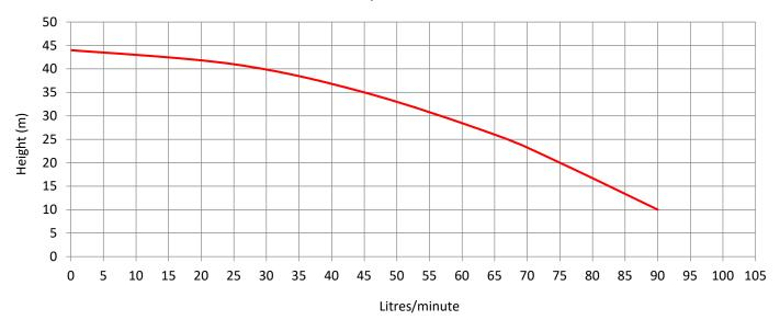
**NOTE:** The above Performance graph is measured at pump outlet and based on factory test conditions. Actual performance onsite may differ due to piping and fixture sizing and layout
